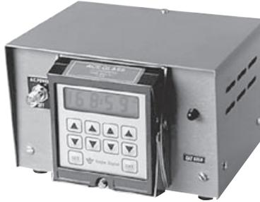
**FRONT PANEL:** Push button ON/OFF AC power switch at left, center module with digital display at top, four sets of increment/decrement arrow push pads, SET<sub>1</sub> and SET<sub>2</sub> push pad lower left, ENT push pad lower right, and red time-on output light at extreme right.
